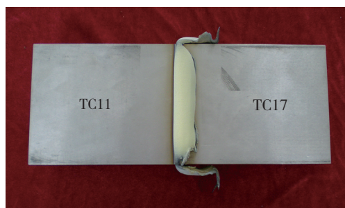
图1 焊接接头的外观形貌 Fig.1 Welding joint appearance
